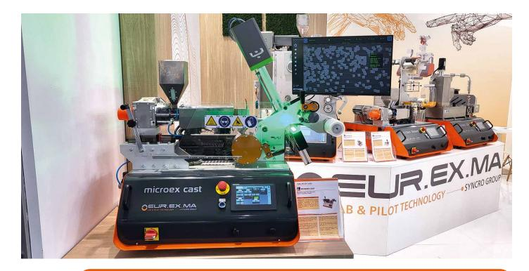
CAST FILM lines are designed for the quality control of polymers, compounds, masterbatches, and recycled materials. The film samples can be used for testing of mechanical properties, processability of polymers, color matching, and visual control of defects.
