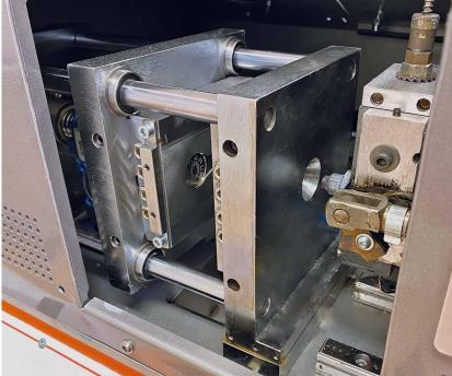
INJECTION MOULDING line is designed to test colours, polymers, and additives. It can also be used to prepare specimens for analytical purposes with low waste and energy consumption.
