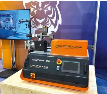
COMPOUND lines are designed to test different formulations of compounds or small batches of additives and color masterbatches with low cost and waste.
