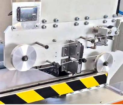
3D lines are used for the production of 3D printing filament. They can process standard materials such as ABS, PLA, PE, TPU or, if equipped with a double cooling system, several kinds of technopolymers.
