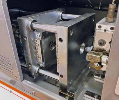
INJECTION MOULDING line is designed for the testing of colors, polymers, additives and to prepare specimen for analitic purposes with low waste and energy consumption.
