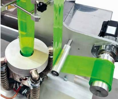
BLOWN FILM lines are designed to create samples of tubular film in different scales for packaging purpose. They are designed for the testing and quality control of different materials and polymers, virgin and recycled.
