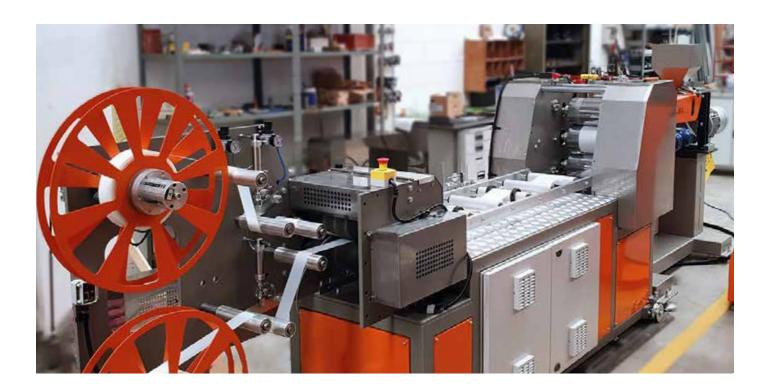
FOIL/SHEET lines are designed for the quality control of compounds and recycled materials. The samples can be used for mechanical properties testing, visual control of defects, processability of polymers and thermoforming.
