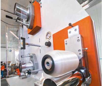
MELT SPINNING line is designed for the creation of continuos filament and Full-Drawn Yarn samples used to test several kinds of polymers.
