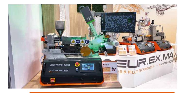
CAST FILM lines are designed for the quality control of polymers, compounds, masterbatches, and recycled materials. The film samples can be used for mechanical properties testing, visual control of defects, processability of polymers and color matching.
